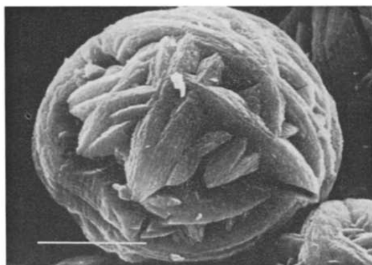
Fig. 3 (left). Crystallite ball of sample 31-01, heated to 1000°C for 2 hours. White line marks 5 \mu\text{m} .
